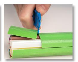
Designed with slim safety heads and high carbon steel blades, this microduct sheath is perfect for slitting the sheaths off microduct bundles to access the microducts inside. This sheath also features the following:
